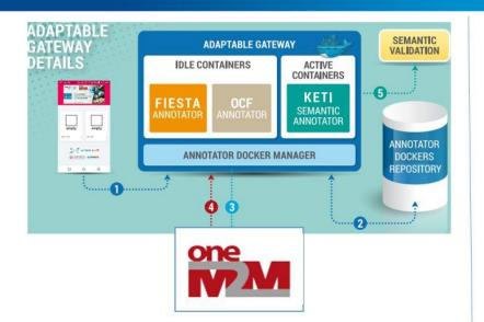
A container transforming oneM2M semantic data into data annotated with FIESTA ontology will be dynamically loaded in the morphing gateway
