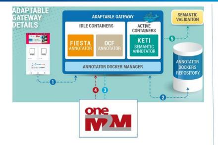
A container transforming oneM2M semantic data into data annotated with FIESTA ontology will be dynamically loaded in the morphing gateway Wrongly annotated semantic data are not able to be retrieved from the semantic repository. In order to prevent such "rubbish" in the repository, not validated data are stopped by the semantic validator
